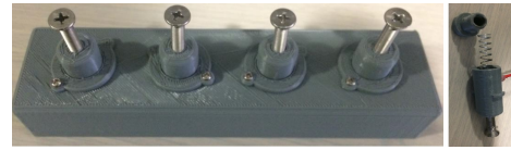
Figure 5. (Left) Assembled electrode arrangement. (Right) Electrode with spring mechanism.
