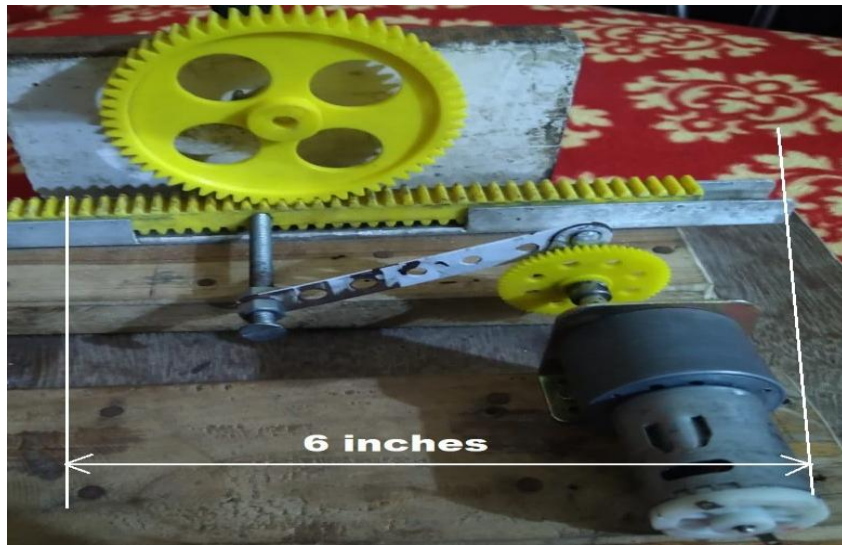
Figure 10 – Proposed ERS based wiper system for automobile
