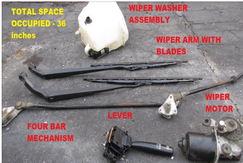
Figure 8 – Various parts of the conventional wiper assembly
