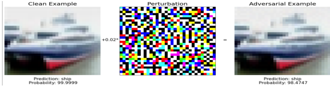
FIG. 12: Illustration of FGSM method for efficiently generating adversarial examples. Note that, we are essentially try to perturb the image along the direction of most likely misclassification with a magnitude \epsilon .
