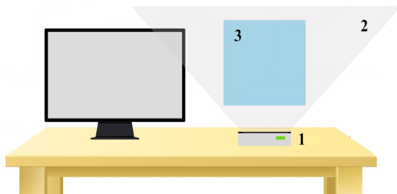
Figure 5. Leap Motion: field of view and interaction box.
