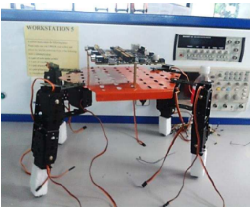
FIG 3.3 JOINTS USING U-BRACKETS FOR THE ROBOT LEG
