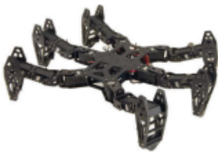
FIG 5.4 ALUMINIUM STRUCTURE OF THE INTELLIGENT HEXAPOD ROBOT
