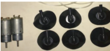
FIG 5.5 SUCTION CUPS AND MOTOR
