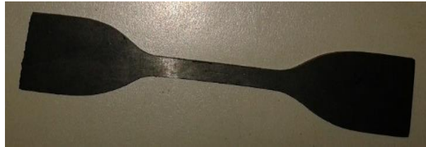
Figure 1. Developed NCAFP composite sample as per ASTM D638-03.
