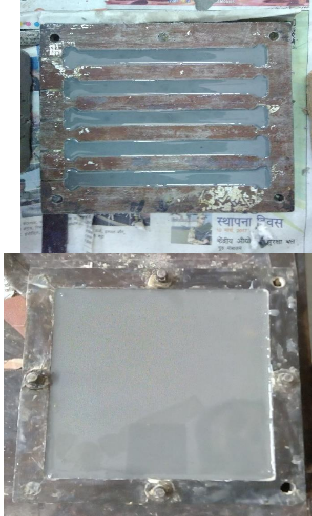
Fig.2 - Shoulder and Plate die with material filled in it.
