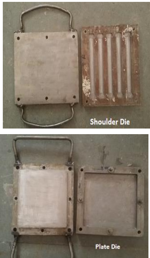
Fig.1- Lower and Upper part of Shoulder Die and Lower and Upper part of Plate Die.
