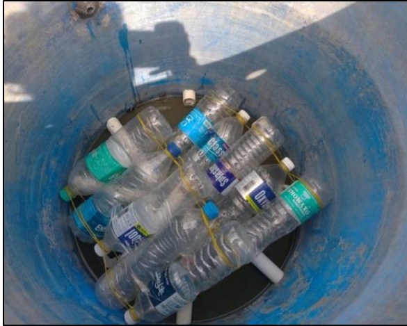
Fig. 2(a) Grid of cross-connected discarded plastic bottles
