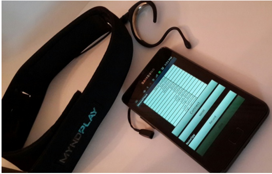
Fig. 14 NeuroSky EEG headset and NeuroPlace mobile app[23].
