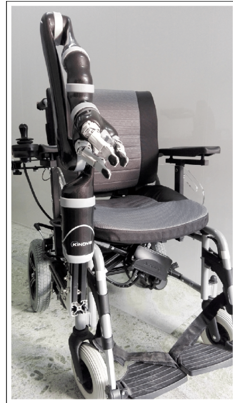
Fig. 15 Robotic Arm mounted on Smart Wheelchair (SWC) with Electroencephalogram[24] (Source : Learning motion primitives from demonstration. Advances in Mechanical Engineering)
