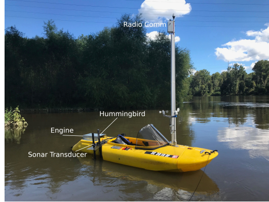
Fig. 4 The AFRL jetyak used during the field deployments. The main controller is the PixHawk that performs GPS-based way-point navigation. In addition different depth sensors are mounted on the boat for surveying operations.
