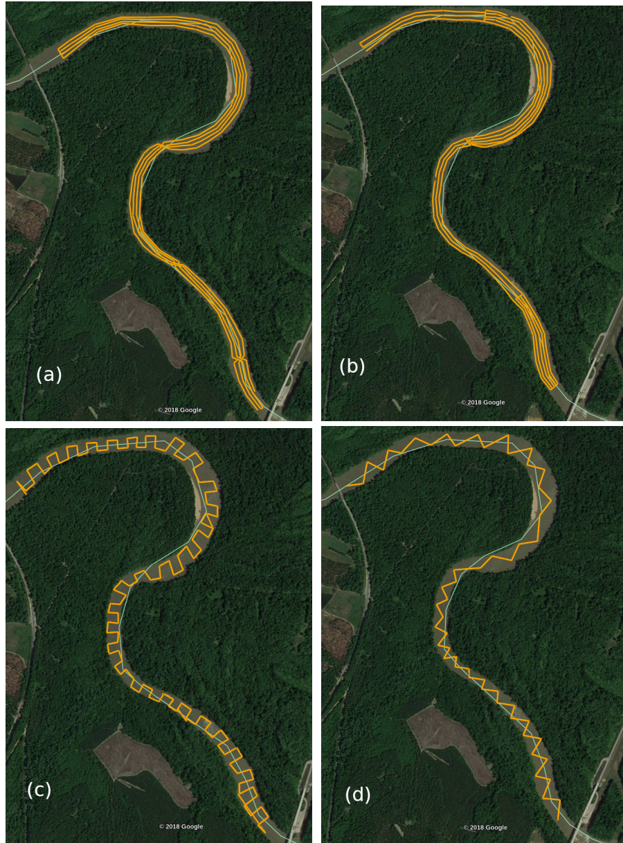
Fig. 7 Way-points of the different coverage patterns executed on the 4.2km long segment of Congaree river, SC. (a) M-cover, (b) L-cover, (c) T-cover, (d) Z-cover
