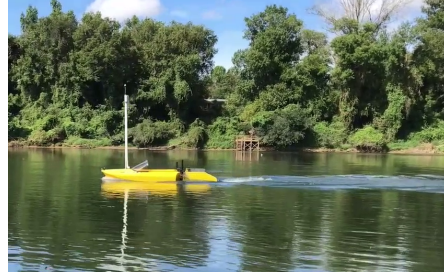
Fig. 1 Autonomous Surface Vehicle (ASV) during coverage operations at the Congaree River.
