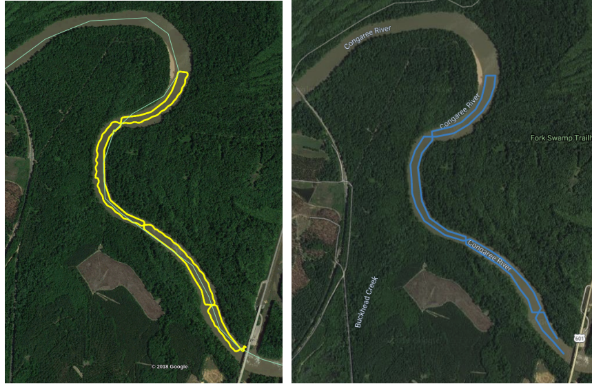
Fig. 5 The way-points generated by the M-cover algorithm (right) with the actual GPS trajectory (left) executed on the 2.76km long river segment.
