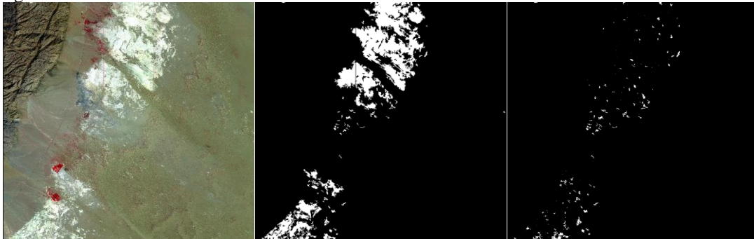
Figure 2: because of edge linear features of big regions, it can effectively eliminate the cloud-like target area by means of geometric fractal dimension. (Figure 2~5 from left to right: Left: cloud area image under detection. Mid: preliminary cloud test results. Right: results after morphological features judgment.)
