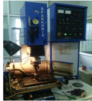
Fig. 2 Specimen of Al-Mg-TiO 2 nano composite and EDM
