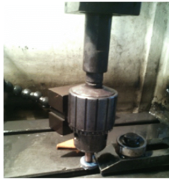
Fig. 2 Specimen of Al-Mg-TiO 2 nano composite and EDM
