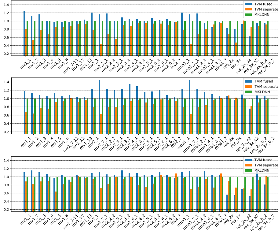
Fig. 4: Throughput comparison between fused and separate kernels without post ops, normalized with respect to MKLDNN. A “TVM fused” result of greater than one indicates our fusion delivers better performance than MKLDNN. Top: Intel i7.7700K (511 GFLOPS); middle: GCP Intel (711 GFLOPS); bottom: GCP AMD (413 GFLOPS).
