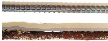
Fig. 6. Actual corrosion ratio of 7,6 % of \varnothing 12 longitudinal reinforcement
