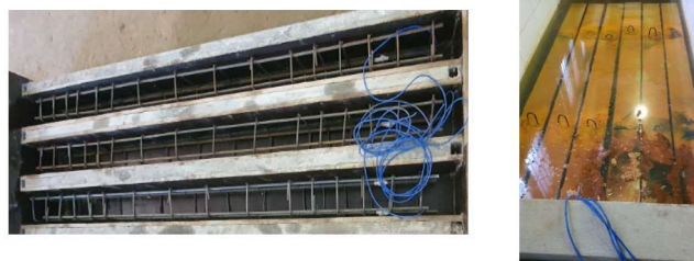
Fig. 3. Electrochemically-accelerated corrosion test
