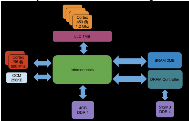
FIG. 3 SIMPLIFIED ZYNQ EG BLOCK DIAGRAM
