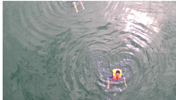
Fig. 6: SeaDronesSee APH-YOLOv7t detection (with persons in blue boxes)
