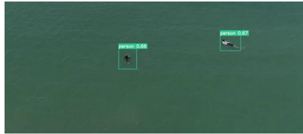
Fig. 5: Mobdrone APH-YOLOv7t detection (with persons in green boxes)
