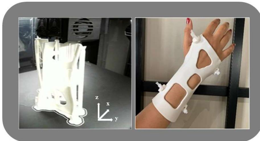
**Figure 1.** 3D printing of arm splint.
