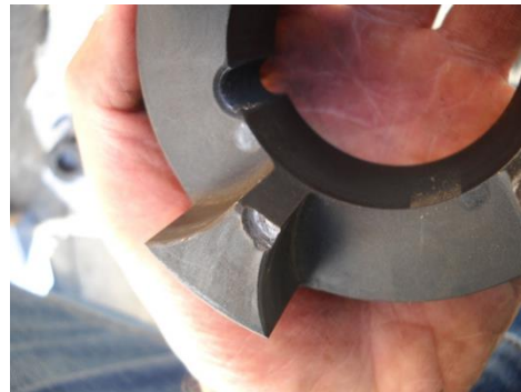
9. Figure. Shaft coupling damage.
