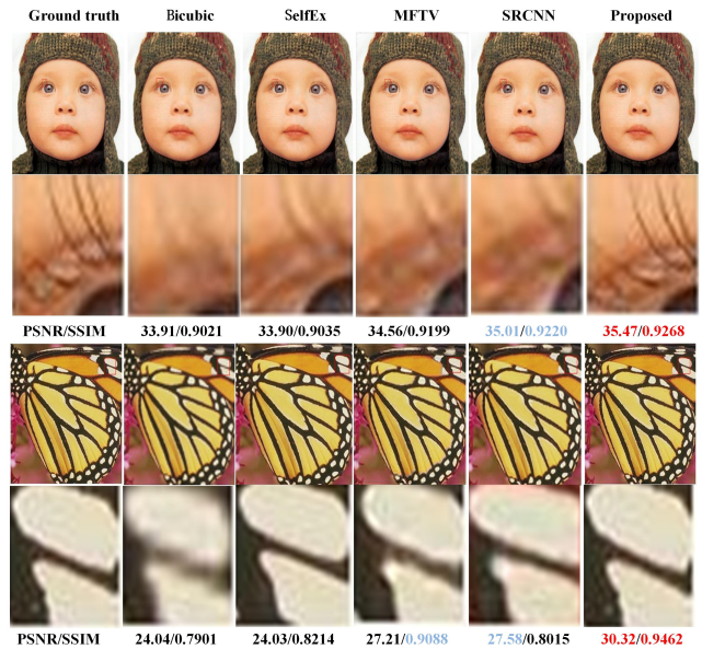
Figure 6. Qualitative comparison. The first row shows image “baby” (Set5 with scale factor \times 3 ). The second row shows image “butterfly” (Set5 with scale factor \times 3 ).
