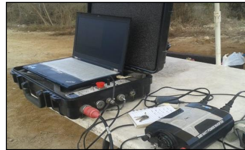
Fig. 1, Well analyzer and computer Source: Pacifpetrol S.A., 2018
