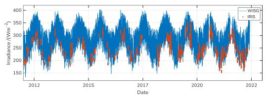
FIGURE 1 Atmospheric longwave irradiance measurements at PMOD/WRC from the WISG (blue), and during cloud-free nights with the IRIS radiometers (red) over the period 2011 to 2022.
