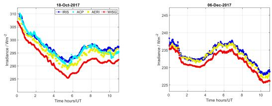
FIGURE 3 Downwelling longwave irradiance measurements from IRIS (blue), ACP (magenta), AERI (yellow), and pyrgeometers traceable to the WISG (red) at SGP for 18 October 2017 (left) and 6 December 2017 (right). The IWV was 11.2 mm on 18 October and 5.3 mm on 6 December.
