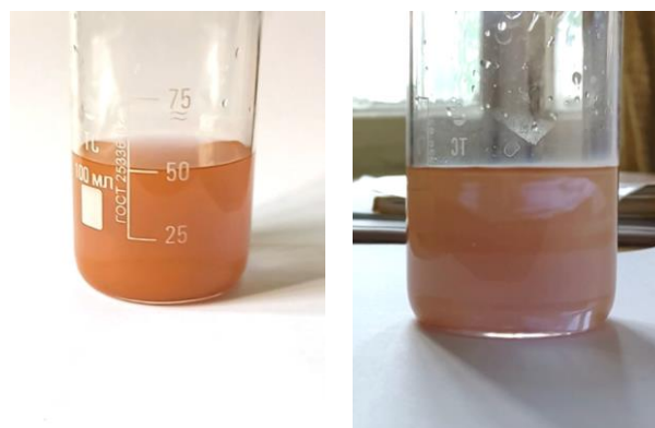
Fig. 2. The image of the gold sol that was obtained using hydrogen peroxide as a reducing agent.
