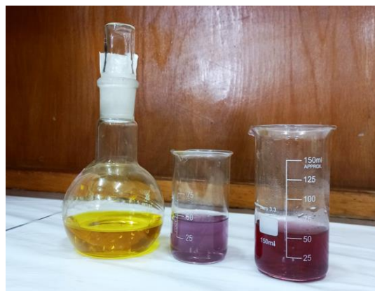
Fig. 1. The images of test objects: on the left we can see the solution of hydrogen tetrachloraurates (III) and in the center and on the right we can see colloidal gold solutions.
