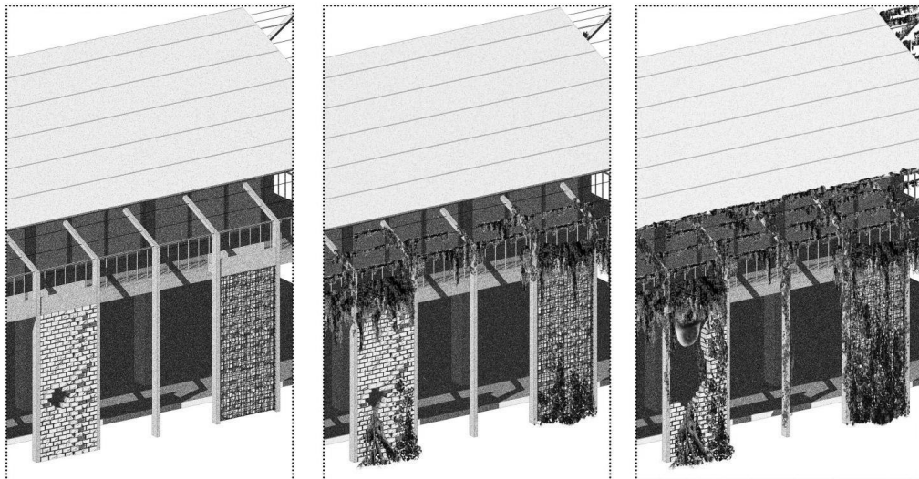
Fig 4. Mortar as a bio-receptive element and Brick protrusion to control biological colonization (Aswin Senthil 2021)
