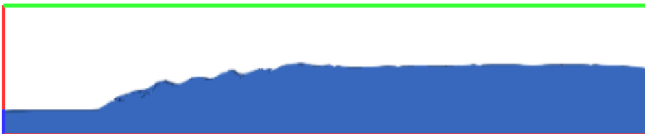
Figure 8: Numerical setup of the hydraulic jump. Off plane boundaries are symmetries, on the bottom left-hand side is the inlet, red denotes a wall and green a pressure outlet.
