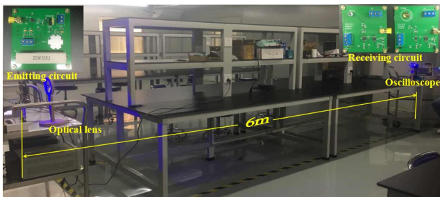
Fig. 3. The test platform. The distance is from 1m to 6m.
