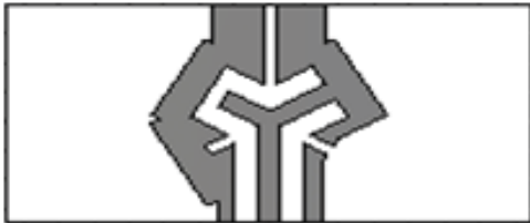
Fig. 6. Simulated prototype of co-planar waveguide to CPS transition based double-Y balun
