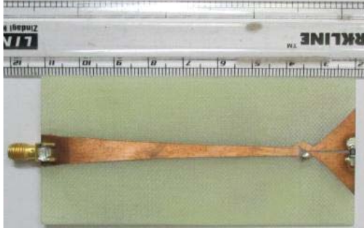
Fig. 11. Bottom view of the fabricated feed structure
