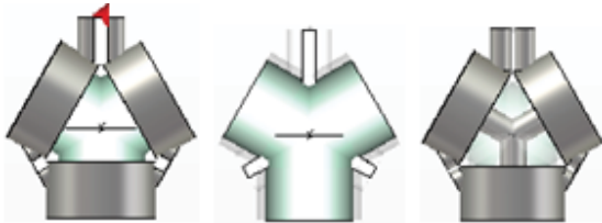
Fig. 7. Simulated prototype of co-axial transmission line to twin wire transmission line transition based double-Y balun
