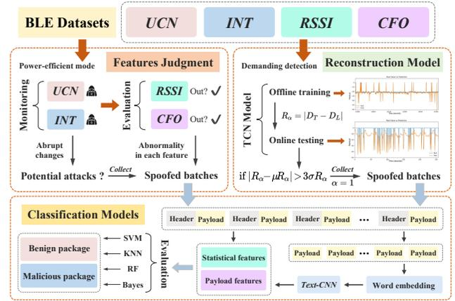
Figure 2: The workflow of BLEGuard detection mechanism.
